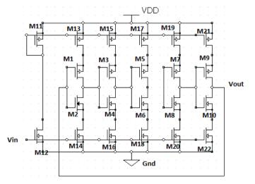
Figure-1: Current Starved Voltage controlled oscillator
