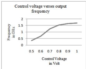
Figure 5: Graphical representation of Control voltage verses output frequency
