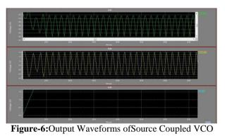
When we applied control voltage 1.4V to 1.8V variable, the Oscillation frequency of the designed source coupled VCO ranges from 307.69 MHz to 425.53 MHz, When we apply control voltage below 1.4V source coupled VCO generates non-linear oscillations. Table II gives the characteristics of the source coupled VCO i.e. control voltage (V) Verses frequency (MHz).
