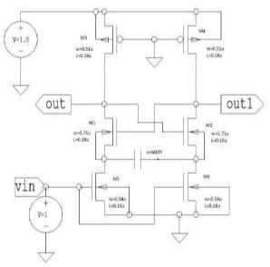
Figure-3 Schematic of Source coupled VCO
