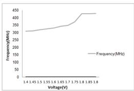
Figure-7Frequency (MHz) Verses Control Voltage (Volt)
